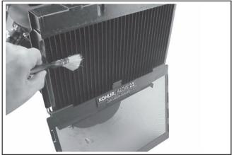
Figure 21. Clean Radiator Cooling Fins and Screen.
